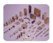
SmCo magnets (Samarium Cobalt) have also a very strong magnetic field. They tend to resist demagnetization extremely well. Unlike Neodymium magnets, it is also very corrosion resistant. SmCo magnets can operate at higher temperatures up to 300°C and are widely used in applications in which higher operating temperature and higher corrosion and oxidation resistance are crucial. The temperature coefficient of remanence is usually less than ±0.05%.
